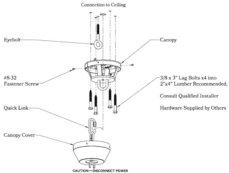
Always shut off power when installing or repairing this (or any other) electrical appliance. Failure to do so may result in severe injury or death. This product must be installed in accordance with applicable installation codes by a person familiar with the construction and operation of the product, and the hazards involved.
